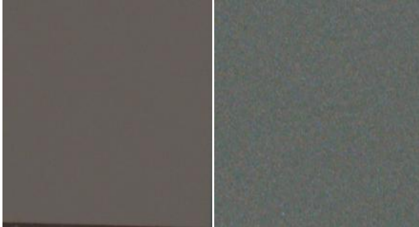
Figure 6. Comparison of Canon EOS 600D (T3i) at ISO 100 (left) and Kodak Portra 160NC (right). The left image was generated directly from the RAW image with minimal image processing: white balance, demosaicing, color matrix and gamma curve. It is not the JPG out of the camera, in particular there is no noise reduction.
